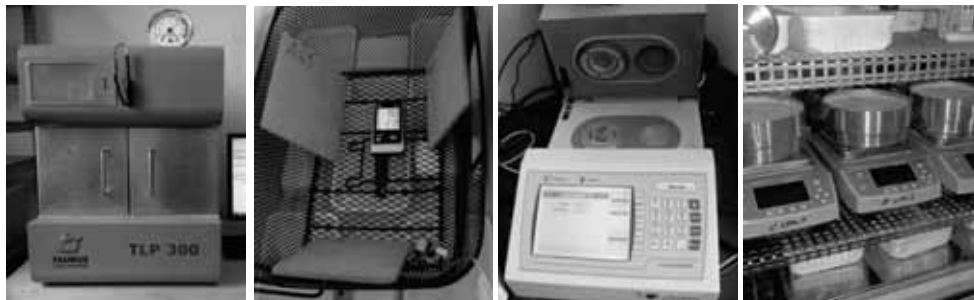
Figure 3. Left to right: Taurus guarded hot plate apparatus; Sorption curve measurement in insulated chambers; Labmaster-aw instrument; Vapour diffusion measurements.
