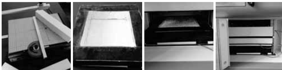
Figure 4. Left to right: Hot wire EPS cutter; EPS stock with Al foil; Perlite filled stock in apparatus; pressed specimen in apparatus with both (hot & cold side) thermocouples on place.
