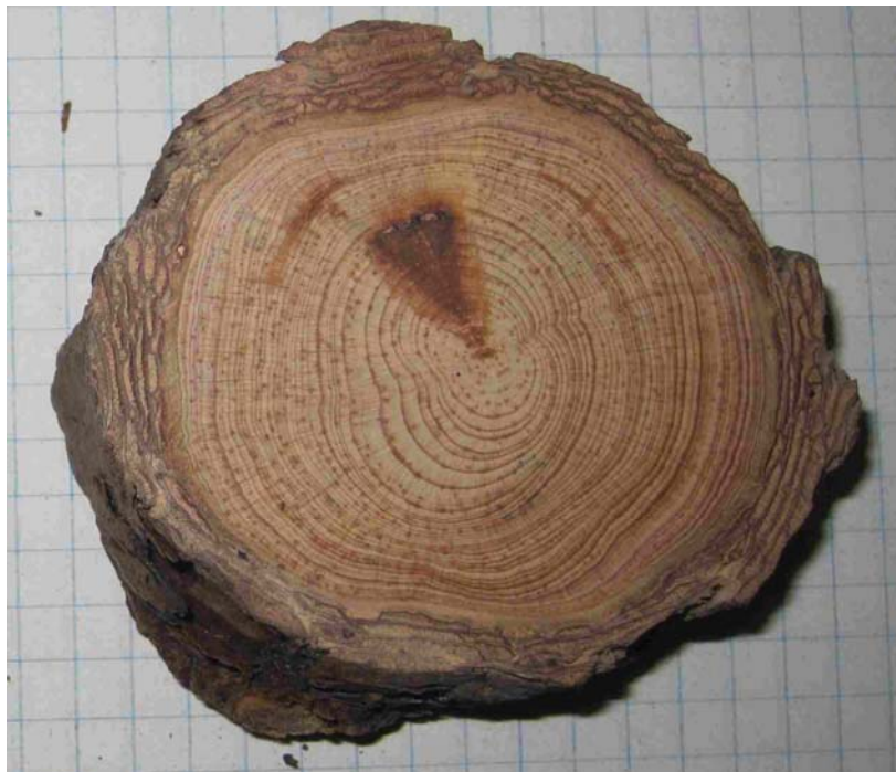
Fig. 19. Initial wide rings were gradually replaced by narrower rings, following the usual age-related decrease of growth of stems. Initial rings bear reasonable amount of latewood, while later, narrow rings have only very thin latewood. Exhumation date can be approached by the first injury only: a black wound, a dark deposit of phenolic substances below, and a single ring of the
