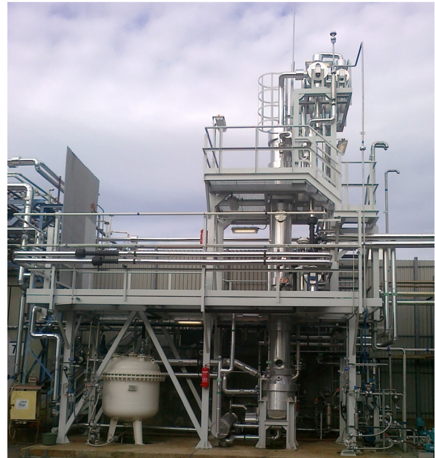
Figure 7: Industrial distillation column for the treatment of chemical wastewaters, from Toth (2015).
