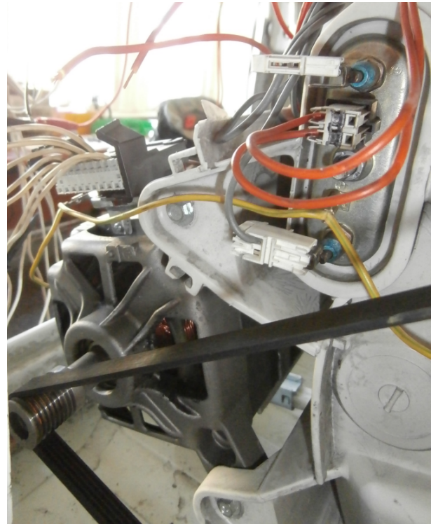
Fig. 4. The main motor and connection of heating body.
