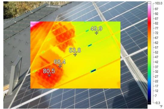
Figure 8: Incorrect measurement due to shaded PV panels
