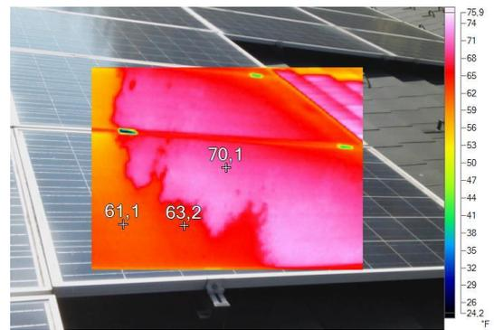
Figure 9: Incorrect measurement due to environmental reflection
