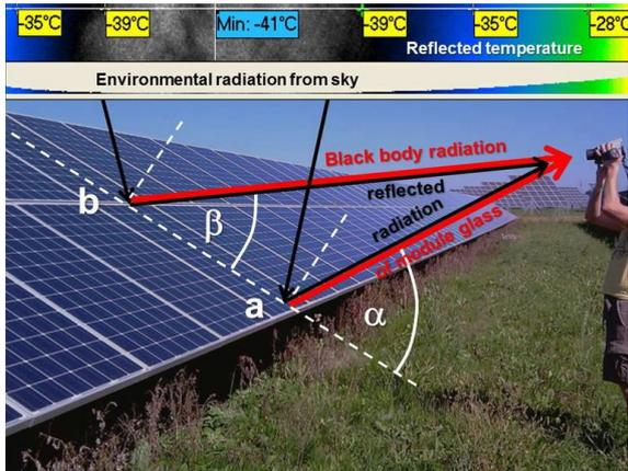
Figure 4: Observation angle for thermal camera measurement [7]
