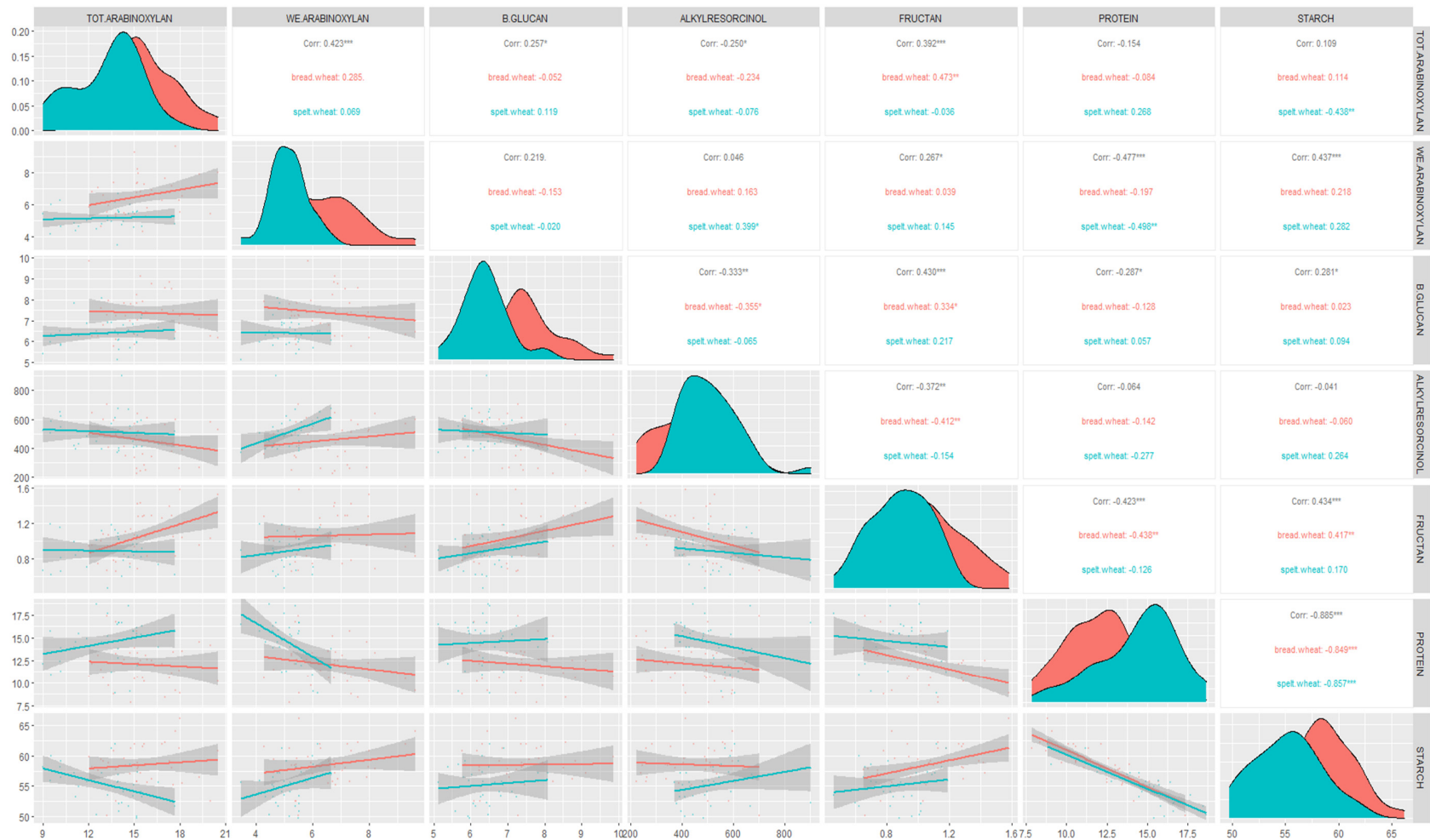
Figure 3. Correlations between the bioactive compound, protein and starch content for bread and spelt wheat. Above the diagonal: the Pearson’s correlation coefficients for bread (red) and spelt (blue) wheat and combined (gray); diagonal: the distributions of each trait for bread (red) and spelt (blue) wheat; below the diagonal: scatter plots with linear regression lines for bread (red) and spelt (blue) and their confidence intervals (gray areas). Correlation coefficients significant for p < 0.001 are marked with ***, those significant for p < 0.01 with ** and p < 0.05 with *. The correlation coefficients that are not marked are not significant.
