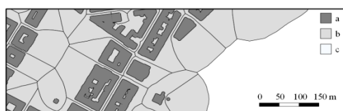
Fig. 2. Examples of lot area polygons. a: building; b: lot area; c: open area
