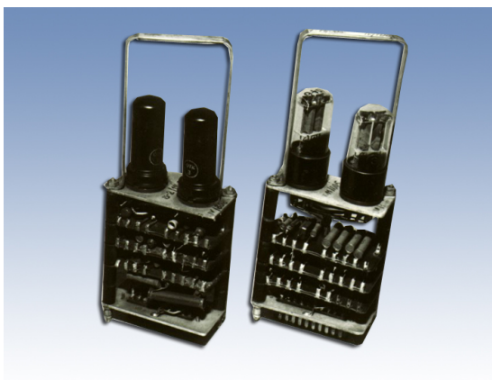
Fig. 2. “The logic units of the M-3 computer, (left) the new developed drum controller-unit, with Hungarian produced long-life tubes, (right) the old unit, original Soviet design with Soviet elements.” ([8], p. 77)
