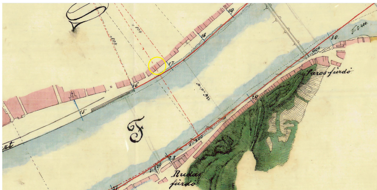
Fig. 9. Map of the part of the river Danube between Buda and Pest with the established regulation line. Yellow circle: site of the excavation in Molnár Street. Red line: planned new coastline. Catalogue of maps of Budapest 267. With the permission of the Budapest City Archives. Archival reference: BFL XV.16.d.241/13
