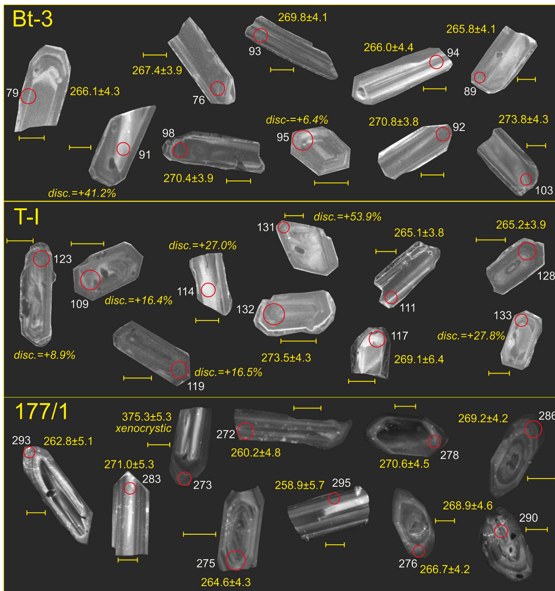
Fig. 8. Cathodoluminescence images of some representative zircon crystals from the samples Bt-3 (crystal-rich pyroclastic rock, southern Transdanubia), T-I (crystal-poor lava-like ash tuff, eastern Pannonian Basin), and 177/1 (deformed ignimbrite, Bihar Mts, Apuseni Mts). Spot IDs, concordant ^{206}\text{Pb}/^{238}\text{U} dates, and discordance values for the discordant dates are given in the figure, and the complete dataset is available in Electronic Supplementary Material 1. The length of the yellow scales beside each zircon crystal is 50 \mu\text{m} , while the diameter of the laser spots (red circles) is 33 \mu\text{m} . (For interpretation of the references to colour in this figure legend, the reader is referred to the web version of this article.)
