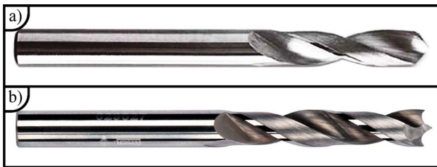
Fig. 3 Illustration of the applied drilling tools: a T1: twist drill, b T2: brad and spur drill
