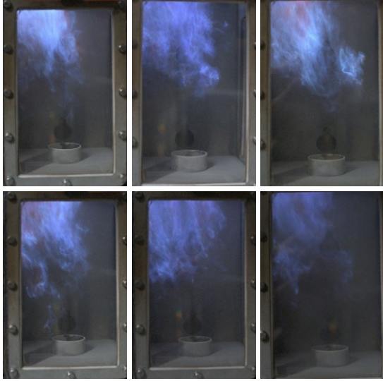
Fig. 2. Flame images of distributed combustion. Top row: T_{ca} = 200\text{ °C} , bottom row: T_{ca} = 250\text{ °C} . Left to right: p_g = 0.6, 0.75, and 0.9\text{ bar} .
