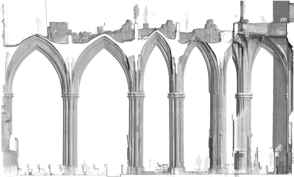
Figure 7. The longitudinal section of the point cloud
