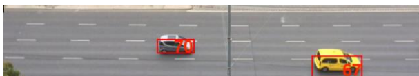
Fig. 1. Detected vehicles can be seen in a selected frame of a measurement recording. The numbers indicate the speeds of the vehicles measured in [km/h].
