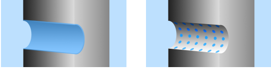
Figure 3: A homogeneous (left panel) and a localised (right panel) charge distribution (in blue).
