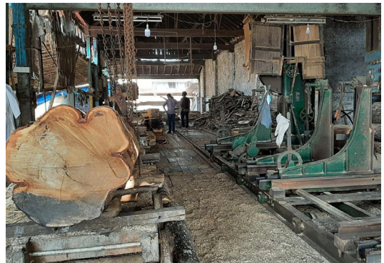
FIGURES 2–3. One of the oldest existing timber mills of Kallai still operating with machines made in Belgium (Brenta bandsaw)
