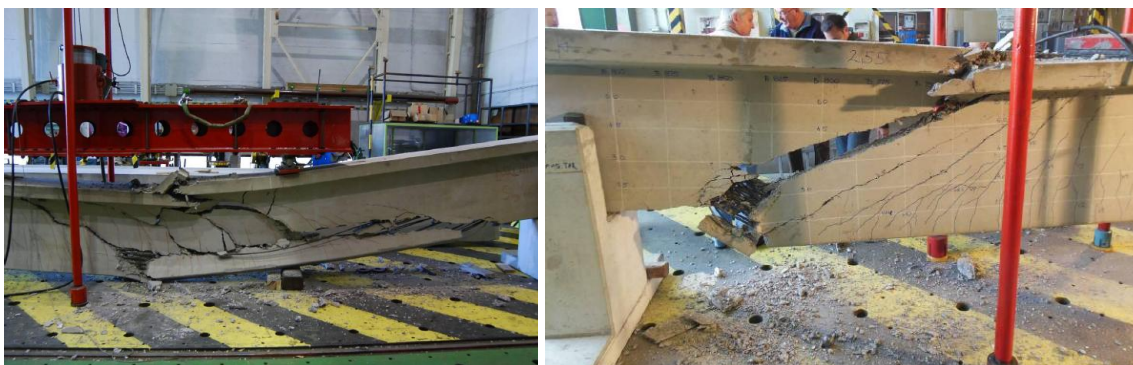
Fig. 3 Bending (left) and shear (right) failure
