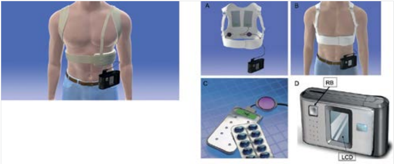
FIGURE 1. Wearable cardioverter-defibrillator/Zoll Life Vest® (A), (B) Garment with 3 defibrillation electrode pads (apex-to-posterior defibrillation) with 4 sensing electrodes, accelerometer in front defibrillation pad; (C) blue colored gel patches; (D) control box. Adapted from Ref 34
