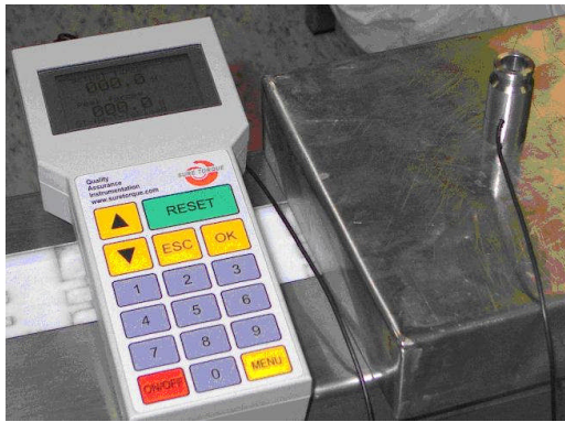
a/ closing force measuring instrument
