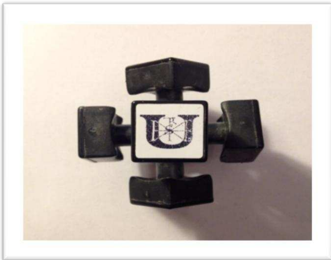
1. Illustration: „Skeleton” of Rubik’s Cube, rotateable, but immovable mid cubes, Source: self-made.
