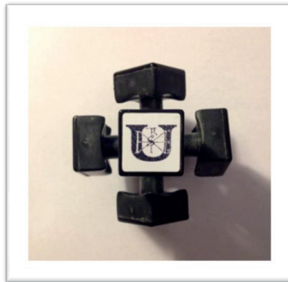
Figure 34: The “skeleton” of Rubik’s Cube is made up of rotatable but immovable middle cubes
