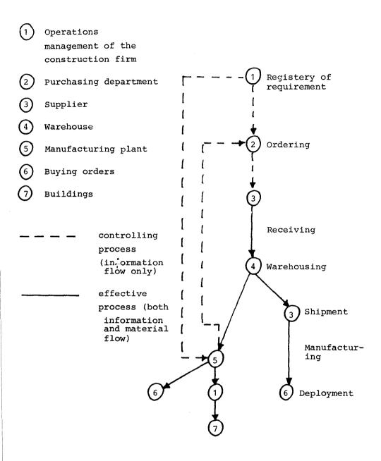
Figure 2 - The general processing flow - ch**ar**t of the items
