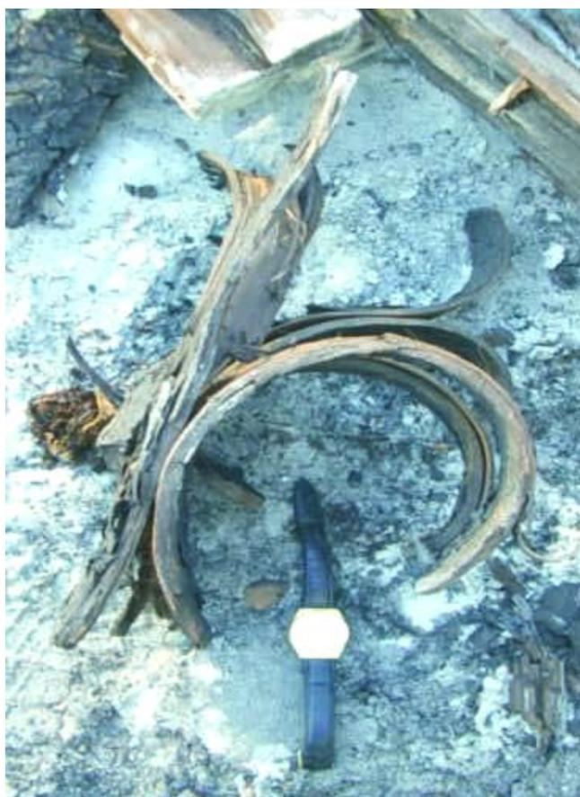
Fig. 14. Peeled-of fragments of trunks are curled while on sunshine due to low resistance of cellulose-poor degraded wood to tensile stress of evaporating water.
