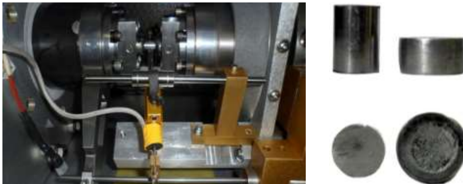
Fig. 2 The experimental setup for cylindrical upsetting
