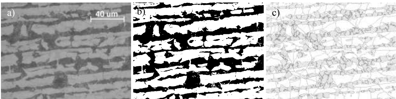
Fig. 2, Development of banded pearlite structure by using a microscopic image (a, grey image [6], b, detected binary image, c, structure to the real ones)
