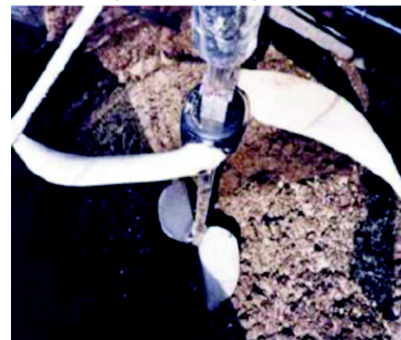
Figure 3. Combination of vertical bladed and propeller stirring fans [5].
