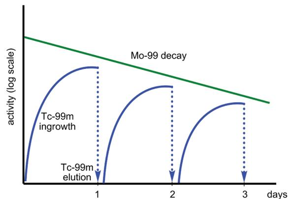
**Figure 8.** Relative activity of Mo-99 and Tc-99m in the generator over time. Maximum buildup of Tc-99m activity is reached in ca 23 h followed by elution.
