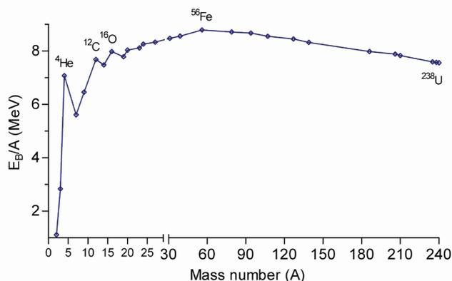
Figure 2. Binding energy per nucleon as a function of mass number.
