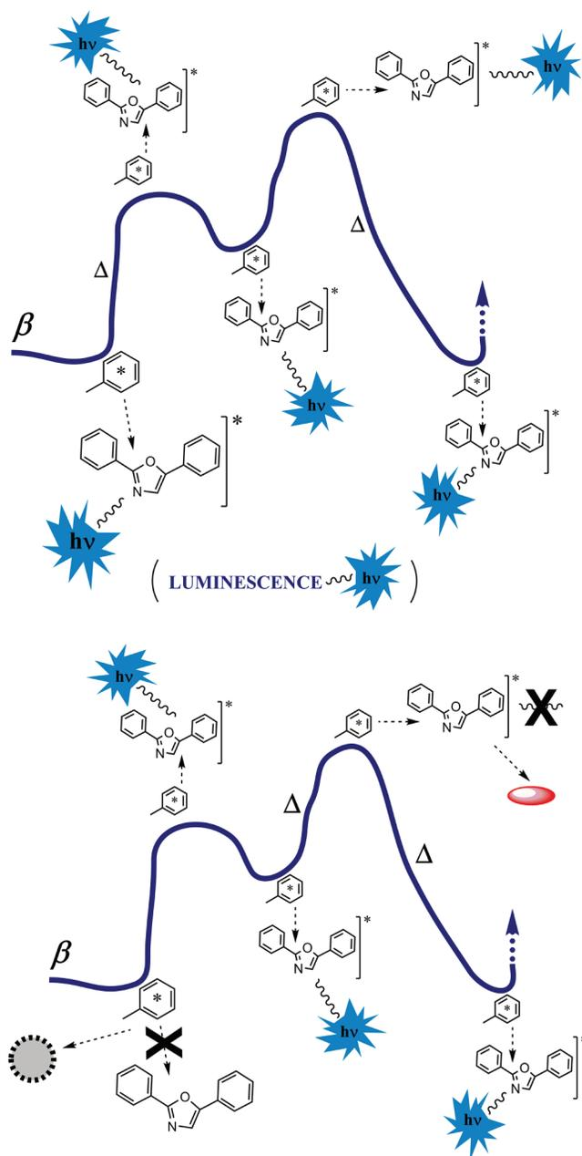
**Figure 5.** (A) Liquid scintillation in toluene solution in the presence of the scintillator 2,5-diphenyl-1,3-oxazole (POP). (B) Points of interference caused by chemical, photon and color quench are indicated.
