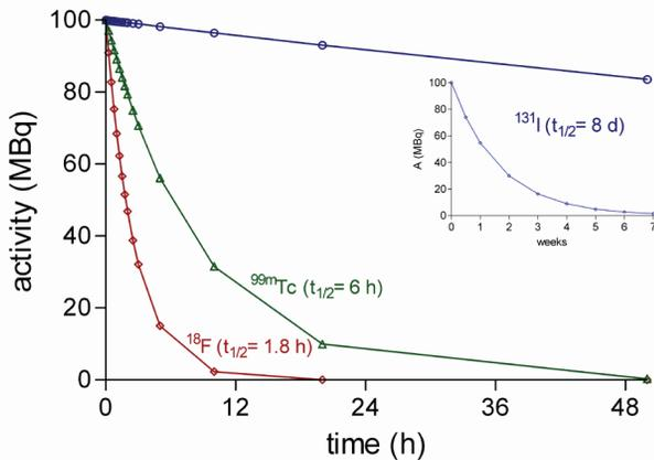
Figure 3. Decay of F-18, Tc-99m and I-131 over time.
