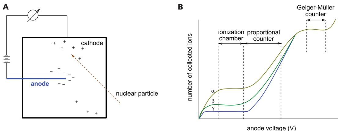
**Figure 4.** (A) Schematic representation of a gas-filled ionization detector. Electrons and cations are produced by the ionization of the filling gas exposed to ionizing radiation. Electrons collected by the anode produce a current which depends on the type and energy of the particle and also on the applied electric field. (B) The relationship between the pulse size produced and the potential applied across the electrodes.
