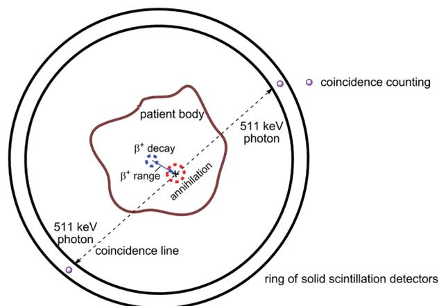
**Figure 6.** Detection of annihilation photons in PET.
