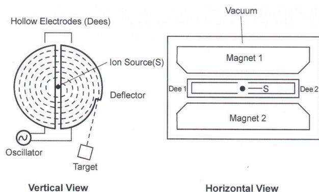
**Figure 7.** Schematic diagram of a cyclotron.(Kowalsky et al. 2011) The trajectory of the accelerated particle is represented by a dashed spiral. Repeated application of accelerating voltages to ions by the hollow electrodes (dees) accelerates ions to high velocities.
