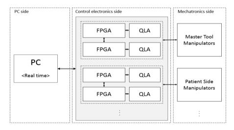
Figure 3: Schematic representation of the hardware structure Workstation [32].
