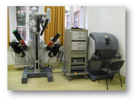
Figure 4: The da Vinci Surgical System and the da Vinci Research kit. System components: Patient Side Manipulators (left), the dVRK controller (middle) and the Master Tool Manipulators (right).
