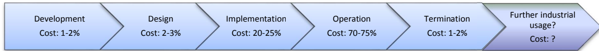
Figure 4 Lifecycle of a large research infrastructure with the average costs for phases. (Based on G7, 2015)
