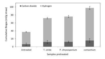
Fig. 4. Cumulative biogas produced after 7 days of fermentation by the untreated, T. viride, P. chrysosponium and a combination of these two fungi species. The results are expressed as mean  $\pm$  standard error of duplicate samples.
