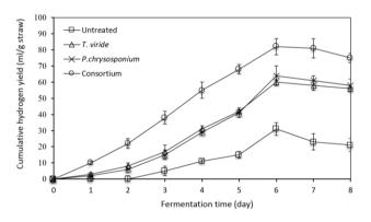
Fig. 3. Cumulative hydrogen produced by the untreated fungi-treated samples. The results are expressed as mean  $\pm$  standard error of duplicate samples.
