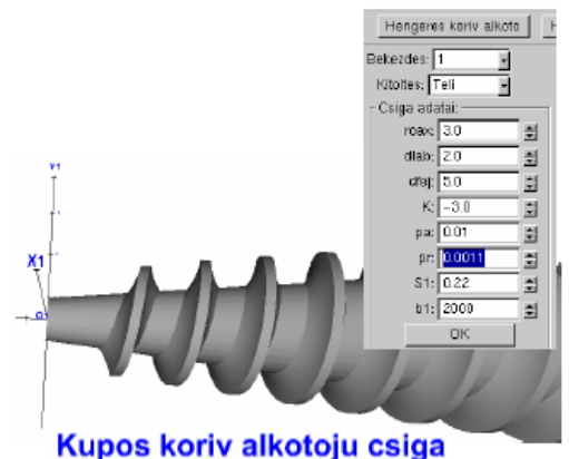
Fig. 9 The conical worm with arched (circle) profile in axial section
