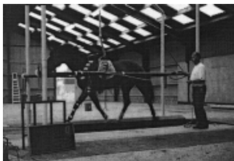
Fig. 1. A photograph taken near (left) to the place of recording. The horse is running on the treadmill and the forelimb is equipped with sensors of CODA visualised with pieces of adhesive tape for better identification in video images. In the left bottom corner the timer device is situated for purposes of synchronisation
