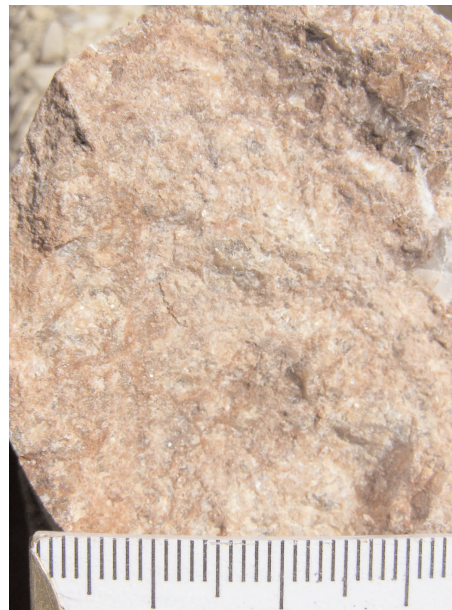
Fig. 3 Close view of reddish-pink granitoid used for shear tests
