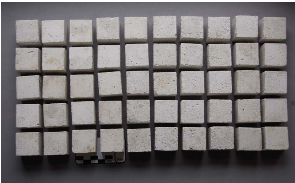
Fig. 1 Repair mortar specimens after being removed from the molds
