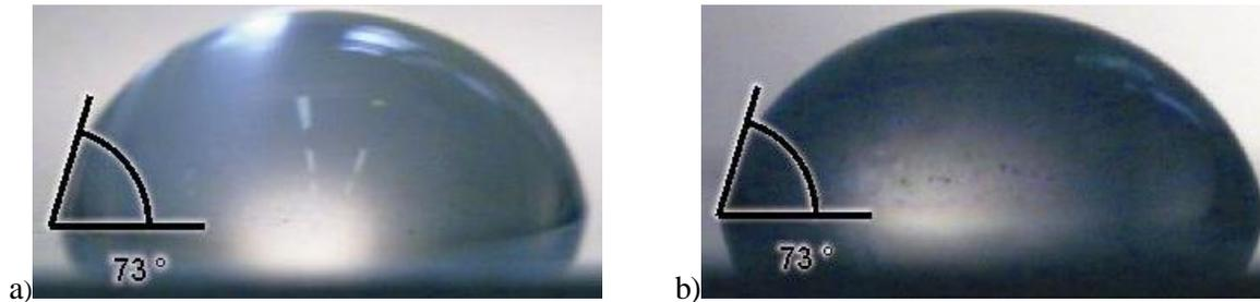
Fig. 13 Photos of the progressive contact angles: a) Polyurethane coated non-electro-polished sheet with a 30 µl drop, b) Polyurethane coated electro-polished sheet with a 30 µl drop
