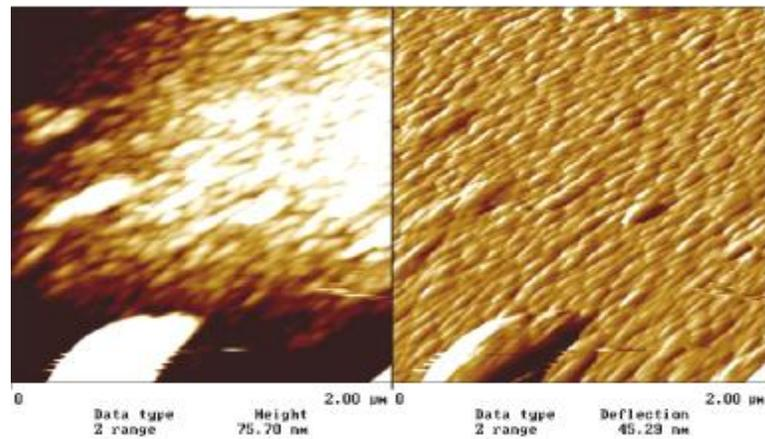
Fig. 5 Atomic force microscopy image of Tecnic Carbostent™
