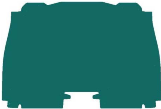
Fig. 6. The optimum blank trimmed for the final shape
