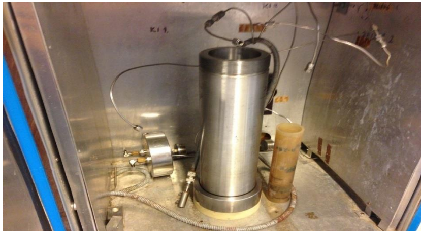
Picture 1. Hassler type core holder
