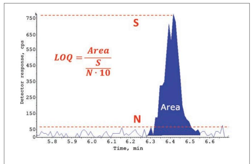
Figure 4. Calculation of the signal-to-noise (S/N) ratio and lowest limit of quantification (LOQ) for a given MRM channel.
