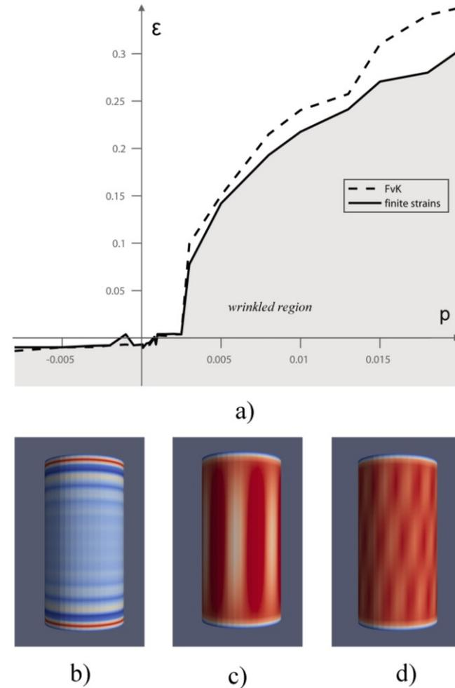
**Figure 4:** Simultaneous axial and lateral loading of a thin, cylindrical shell. a) is the numerically obtained stability boundary of the problem: observed, that at a fixed external pressure there is a critical stretch,  $\varepsilon$  which makes the wrinkled pattern disappear. Also note the quantitative difference between the classical FvK and the model extended to finite strains. Wrinkled patterns around the stability boundary b)  $p = 0.00008$ , c)  $p = 0.0009$ , d)  $p = 0.0025$
