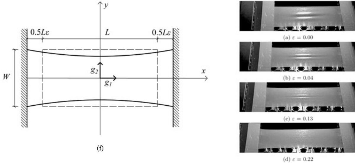
**Figure 1:** Experimental evidence of disappearance of wrinkles for stretched rectangular sheets,  $\varepsilon$  denotes the stretch applied between the clamped edges of the pulled sheet. The material is a 40  $\mu\text{m}$  thick polyurethane tape.
