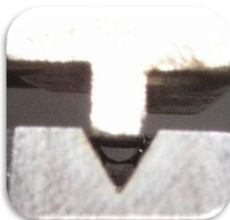
Fig. 3 Crushed stent in the prism
