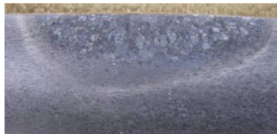
Figure 2. A cross-section of bead-on-plate welded with TIG process; weld penetration less than 3 mm.
