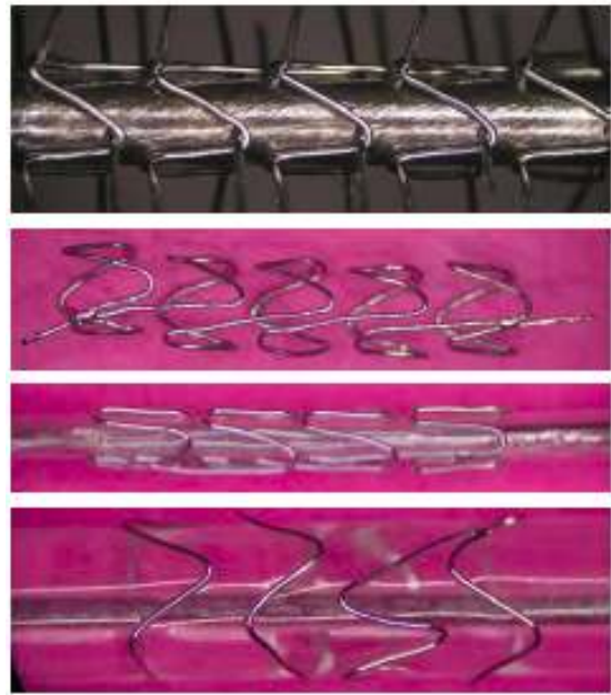
Figure 11: Producing and balloon expansion steps
