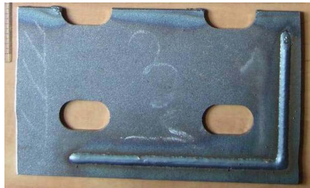
Figure 15. S960QL steel plate no. 3 containing the bead on plate weld.
