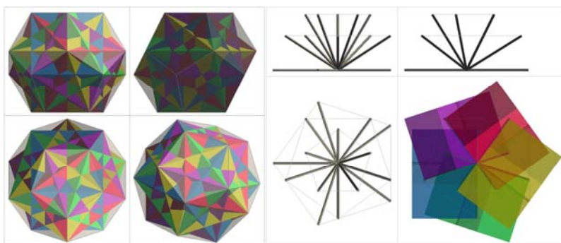
Fig. 2. Five cubes constructed into the Platonic dodecahedron, orthographic views and axonometric projection. Their copies have a common vertex and 15 differently directed edges
