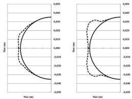
Fig. 7. The 2D geometry of computed accreted ice layers on the surface of the given cylinder (airfoil) of the Global Hawk UAV after 5 minutes flight time. T= -4.2 °C; p = 950 hPa; LWC = 0.5 g/kg; Left: TAS= 50 m/s. Right: TAS= 100 m/s. The blue line shows the ice accretion geometry and the brown one represents the surface of airfoil itself
