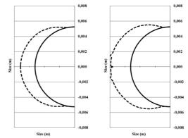
Fig. 8. The 2D geometry of computed accreted ice layers on the surface of the given cylinder (airfoil) of the Skylark-I SUAV after 5 minutes flight time.
