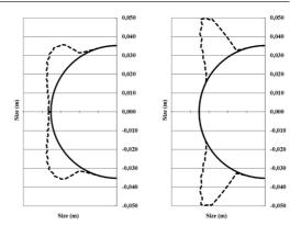
Fig. 10. The 2D geometry of computed accreted ice layers on the surface of the given cylinder (airfoil) of the Global Hawk UAV after 5 minutes flight time. T= -4.2 °C; p = 950 hPa; LWC = 0.5 g/ kg; Left: TAS= 110 m/s. Right: TAS= 130 m/s. The blue line shows the ice accretion geometry and the brown one represents the surface of airfoil itself
