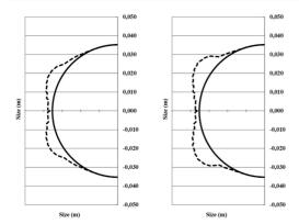
Fig. 9. The 2D geometry of computed accreted ice layers on the surface of the given cylinder (airfoil) of the Global Hawk UAV after 5 minutes flight time. T= -4.2 °C; p = 950 hPa; LWC = 0.5 g/kg; Left: TAS= 70 m/s. Right: TAS= 90 m/s.
