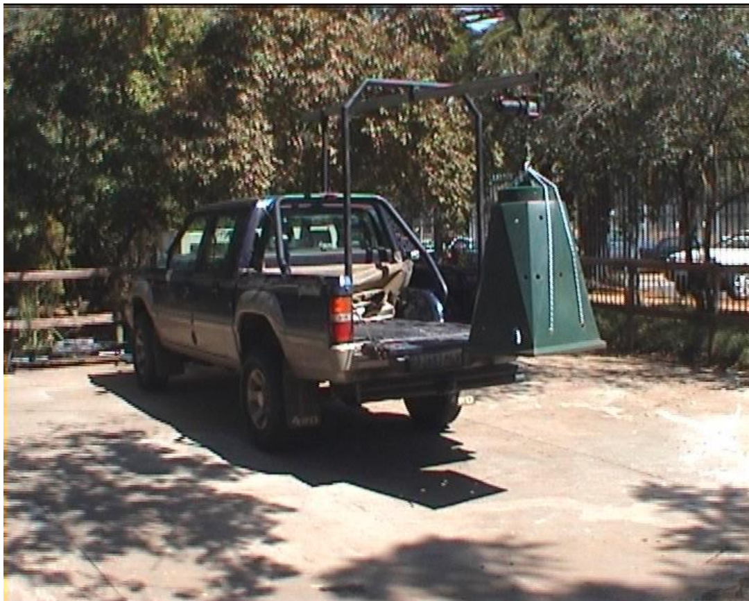
Fig. 4. The truck equipped with the frame
