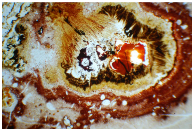
Fig. 11 Contaminated limestone sample from Bed 2 of the Dezső Rezső Valley section, Zengővárkony. It shows the contact zone of the limestone and the basaltic rocks
