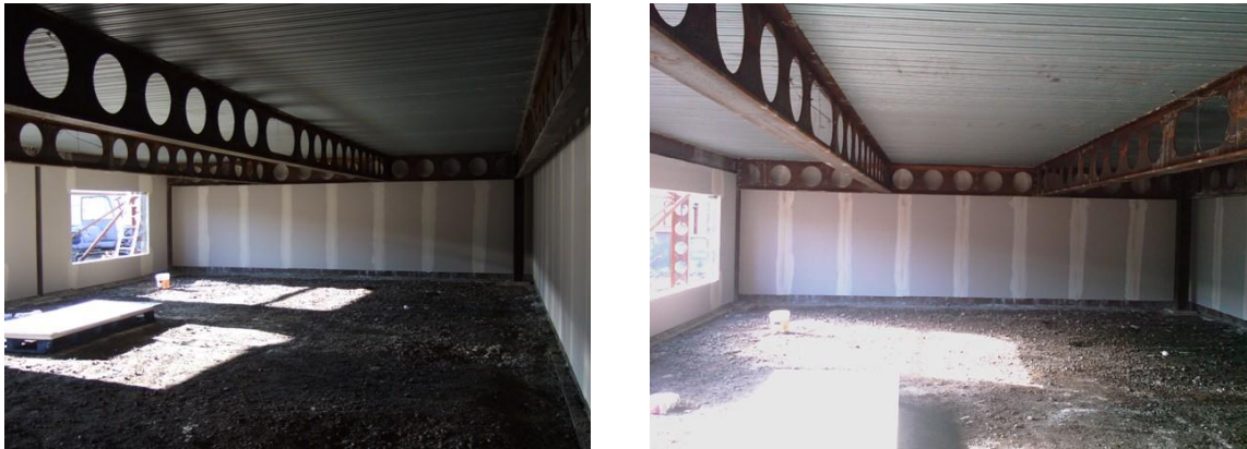
Figure 3.1. Test compartment with long unprotected cellular beams
