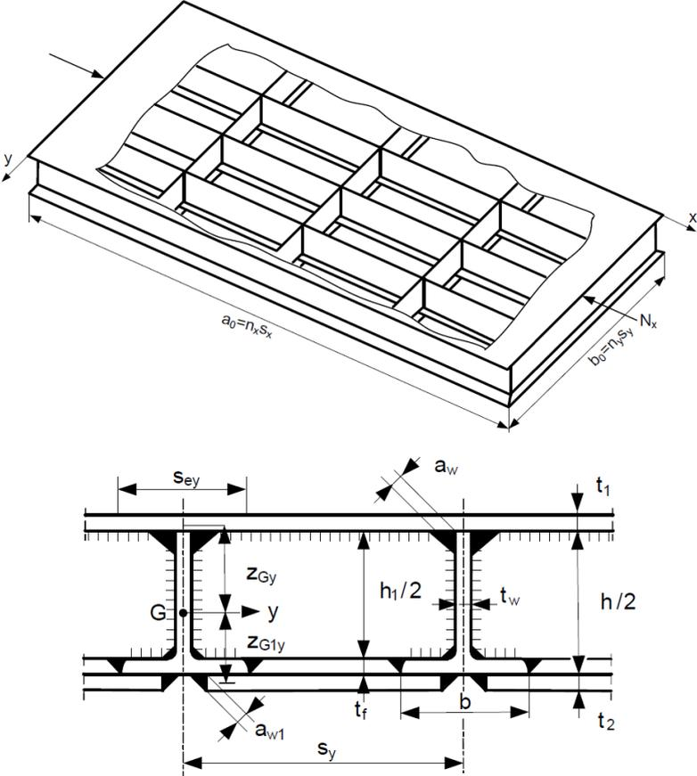
Figure 4. Orthogonally stiffened cellular plate and its cross-section
