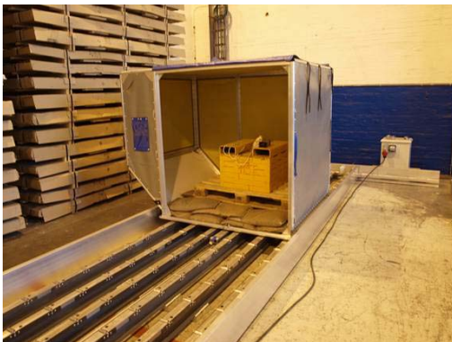
Figure 5. Dynamic testing of actual air cargo container on the rig. (Bode 2016).
