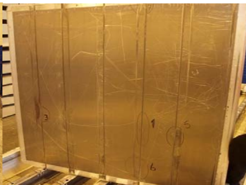
Figure 6. Visible wear lines on the aluminium plate, where the rollers and structure made contact (Bode 2016).
