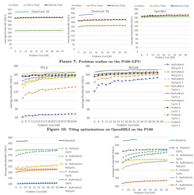
Figure 8: Tiling optimisations on CloverLeaf 2D on the P100 (P-PCI-e, N-NVLink)
