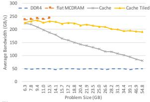
Figure 3: CloverLeaf 2D problem scaling on the KNL
